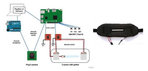
Figure 11-2: Prototype components: Pixy2 CMU (2.1) camera, PixyMon2 software, Arduino UNO, Raspberry Pi 4, L298N motor drivers with 9V power supplies, Pushbuttons, TEC-1-04008 Thermoelectric Cooling Module (light blue) and DK-TEM ES-02 Module (grey) [by fritzing.09.3b] [edited].
