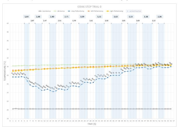
Figure 11-5 Chart I: Visualisation of the recorded cooling process of an active stop command by participant ID046 (blue line). Light blue bars demonstrate the user's perception duration and required difference in relation to the outgoing temperature. [12] p 75
